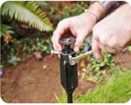
Insert the Anchor Spike Hammer Installation/Removal Tool all the way in the anchor spike socket and tighten the 3 adjusting bolts with a ½ inch wrench on to the flanged portion.
